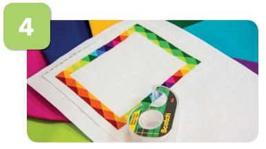
Once the fabric label is positioned where you want it to be, use the tape to secure the label to the bond paper. Ensure the label is correctly positioned. Ensure that ALL four edges of the fabric are completely taped to the paper. The tape is the only stabilizer for the label and it must be well secured or you will get rippled lines of printing.
